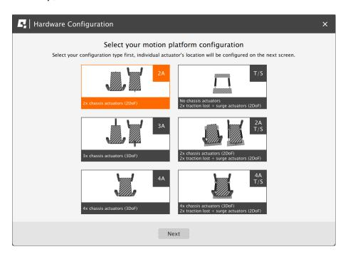
**For QS-210 3DoF set:** Choose the correct layout variant from the list (4 actuators setup).
