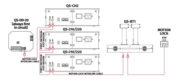
**4.** QS-210 3DoF with a motion platform (**QS-CH2**) and seat belt tensioner (**QS-BT1**).
