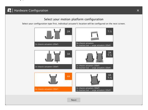
For QS-210 3DoF set with traction loss control (QS-CH2): Choose the correct layout variant from the list (4A+T setup).
