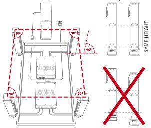
VARIANT 2: Diagonal actuators setup
