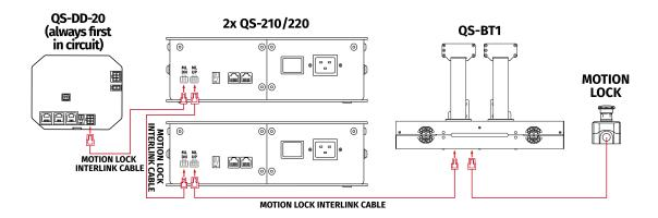
**3.** QS-210 3DoF with a motion platform (**QS-CH2**), seat belt tensioner (**QS-BT1**) and a direct drive steering wheel (**QS-DD-20**).
